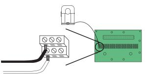
Install the current sensors onto the conductors to be monitored. Sensors can be mounted facing either direction; orientation does not affect meter accuracy. Install E31CT0 on 300 VAC maximum, 50/60 Hz. Install E31CT1 and E31CT3 on 300 VAC max., 50/60 Hz (CE) or 600 VAC max., 50/60 Hz (UL)
