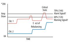
\*Example represents 20 Amp circuit †Configurable time delay for alarm and warning
