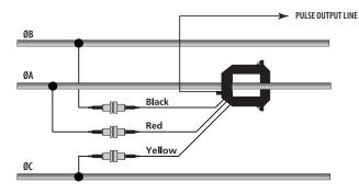
NOTE: Multiply output by 3 for proper kWh indication (Assuming balanced load)
