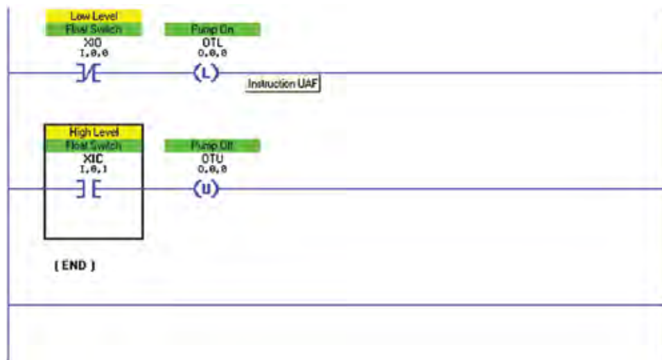
Figure 13: Float Switch control
