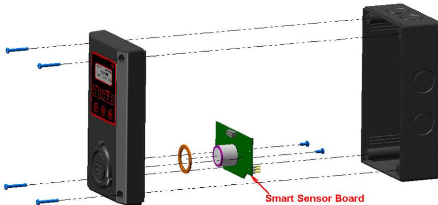
Important: Calibrate the transmitter whenever a component is replaced. But if you replace a smart sensor assembly with a sensor onboard from QEL, you don't need to recalibrate the transmitter, as all the calibration information has been stored in the smart sensor board in the factory process.
