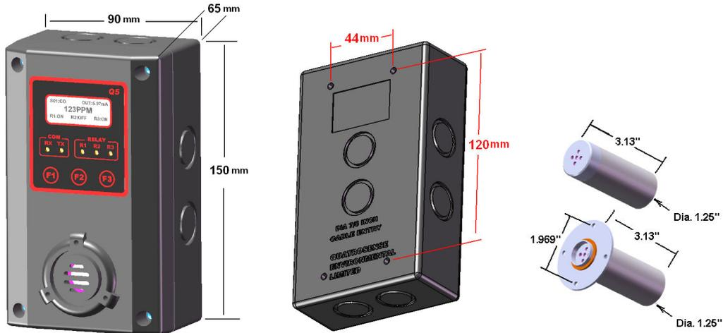
The enclosure is a NEMA 4 rated enclosure and can be wall mounted with 4 screws. To maintain the NEMA rating, it is important that the conduit opening is sealed upon installation.
