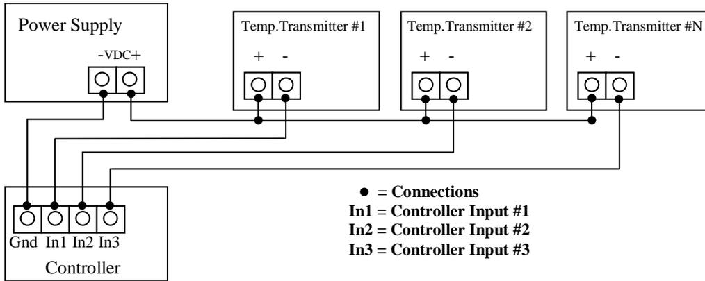
All A/TT and TTM temperature transmitters are reverse polarity protected.
